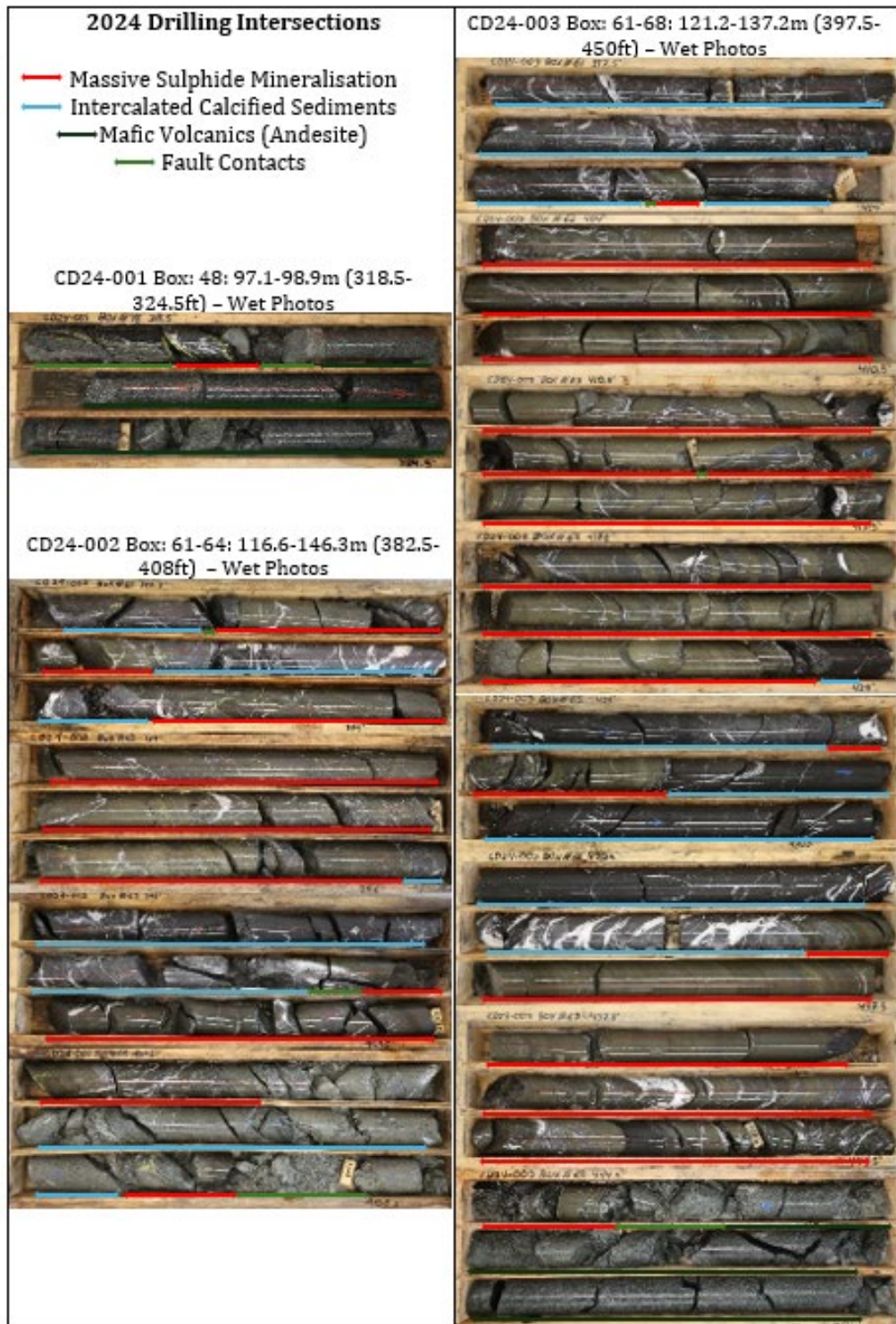
Figure 5. Massive sulphide mineralised intercepts in all core boxes from holes CD24-001, CD24-002 and CD24-003
